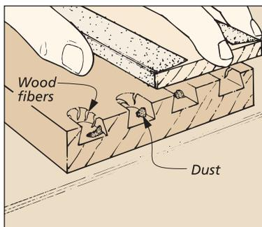
**8** Before testing the fit of the joint, blow out any remaining wood chips and sand off any "whiskers" that are still attached to the pieces.
