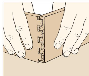
**9** The dovetails should easily fit into the sockets about half way. A couple of taps with a mallet should drive them in the rest of the way.
