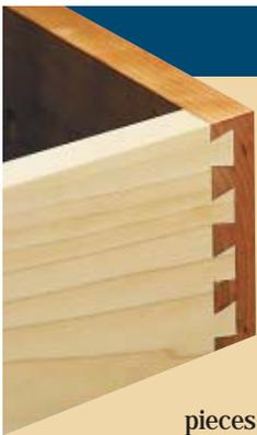
Setting up to rout machine-cut dovetails always involves a trial-and-error effort. There's usually lots of fiddling around with test pieces and adjusting of the jig to get a perfect fit.
