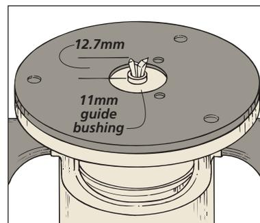
**4** Mount 11mm guide bushing onto router. Then to start with, raise bit 12.7mm from router base. It may have to be adjusted slightly later.
