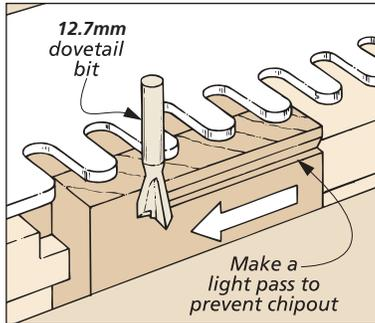
**5** To prevent chipout on the drawer side, start by making a light pass from right to left. This skim cut establishes a clean shoulder line.
