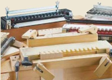
lie in the type of clamping system (some use cams, others use wing nuts), the material used for the template (plastic or metal), and the ease of adjusting the stops.
