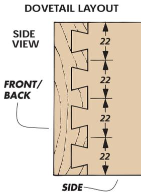
**1** The stops on the ends of the jig are used to create an 11mm offset between the two workpieces and to position them from side-to-side beneath the template. You'll need to adjust each end of the jig independently, since half the joints are cut on the left and half on the right.
