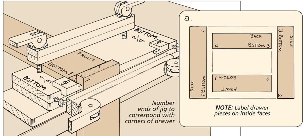
and half on the right side. **Shop Tip:** To help myself keep straight which corner goes where, I also label the ends of the jig, see drawing above.
