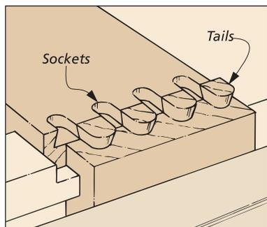
**7** Finally, remove the template (but not the workpieces) and check to make sure that all of the dovetails and sockets are uniform.
