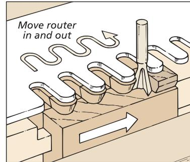
**6** Next, move the router from left to right in and out of the notches. Push the router into each notch until the bushing hits the back of the notch.
