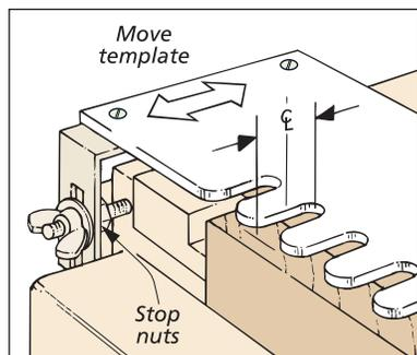
**3** Stop nuts should be adjusted in or out so fingers of template are centred over the "joint line" between the two test pieces.
