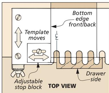
**2** With the test pieces in the jig, adjust the stop so the edge of the front test piece is centred in the first notch or opening of the template.
