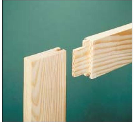
When making a haunched mortise and tenon joint, there's nothing unusual about creating the grooves or the mortises (Steps 1 & 2). Just make sure that the mortises are sized to match the width of the grooves. The tenons are pretty much the same as a traditional tenon too (Steps 3-6). The only difference is the extra shoulder (haunch) on the outside edge.
